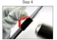
Heat the top section of the Shrink Loop.
