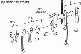
NOTE: Tonnage ratings do not apply when: 1) using jaw blocks with lock screws facing inboard (see drawing C above), 2) jaw angle exceeds 7° or 3) lighter adjustable jaws are used in heavier jaw blocks.
