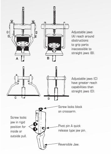
Jaws slide into place along crossarm and may be positioned at unequal distances from the forcing screw for unusual pulling applications.
