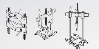
No. J4332 has two sets of drilled holes. One set (A) directly apart, has 1/2"-13 UNC thread, to accept common 1/2" cap screws easily gripped with No. J4018 cap screw jaws (1). A second set (B), diagonally apart, has 5/8"-18 UNF threaded holes to accept Press-N-Pull<sup>™</sup> leg ends (2).
