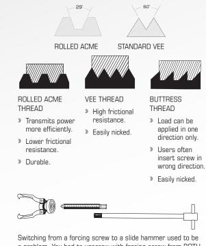
a problem. You had to unscrew with forcing screw from BOTH cross block and adjusting cone and this caused you to lose the set of your jaws. Then you had to "hook-up" all over again. No more! Out comes the screw and in goes the slide rod. You've got a slide hammer puller. The adjusting cone? It stays put...on the cross block.
