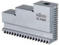
A28 Unstepped Jaw BL, set, diagonally tothing, unstepped, soft, material 16MnCr5
